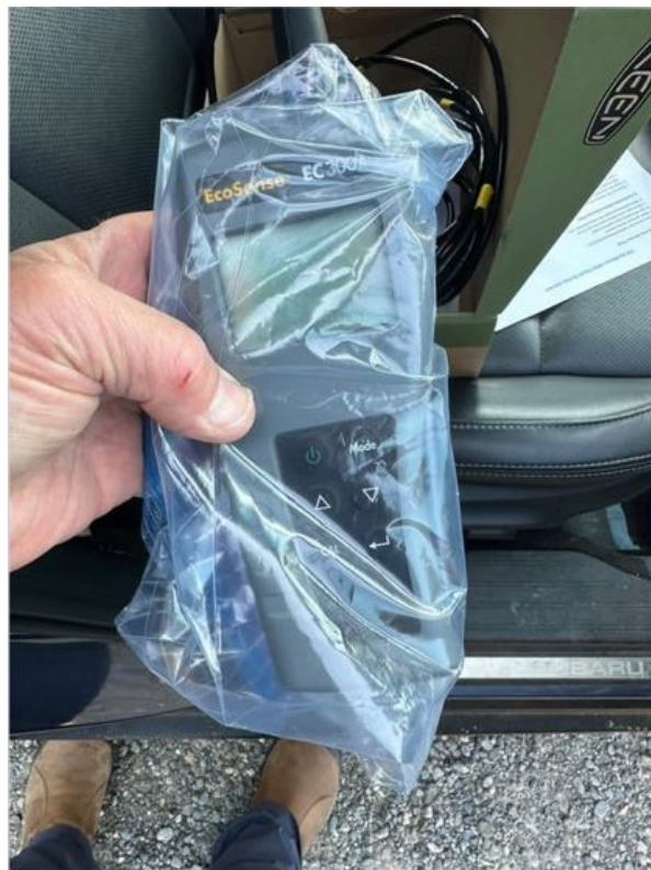
Image 4. Shows simple measures taken by the Lowell Point Team to extend the lifetime of the YSI EcoSense 300As. Courtesy of Doug Palm.
