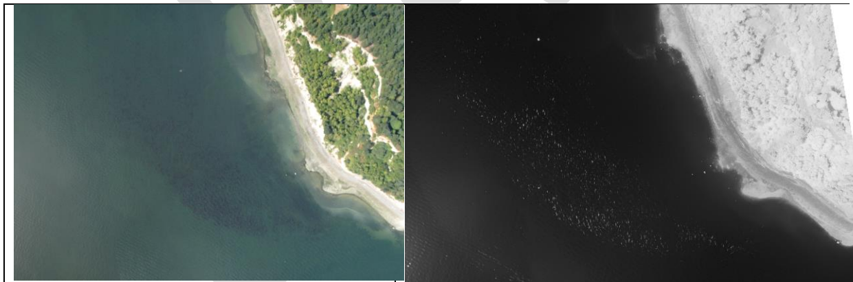
Figure 14. Possession Point bull kelp bed on August 20, 2017, contrasting appearance in visible light (left) with near infra-red (right). Note that nearly all of the kelp is visible at the surface in the near infra-red image. Photos by Gregg Ridder and Vernon Brisley.
