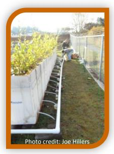
The MRC tested the effectiveness of phytoremediation – the use of plants and soils to remove contaminates from water – to remove heavy metals from treatment plant effluent. Trees were planted in boxes along with one of four different soil types. These "phytoboxes" were watered with effluent from the Coupeville Treatment Plant. The outflow from the phytoboxes was compared with the treatment plant effluent.
